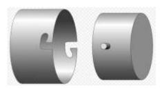
Bayonet mount locking mechanism
