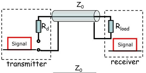
Coax cable has complex impedance Z for signal transmission,  $ReZ=Z_0$
