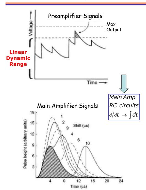
High count rate (relative to pulse length/decay time) can lead to pile up
