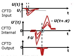
Constant-Fraction Timing Disc.: Corrects for "walk" t(U)  $U'(t) = f \cdot U(t) - U(t + \Delta t)$   $\rightarrow t (U'=0) \text{ independent of } U$   $t(U'=0) - t(U=U_T) \text{ measures } t_R \text{ rise}$ time (here fraction f = 0.5)
