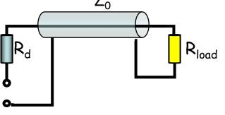
For mismatch,  $R_{load} \neq Z_0$ , reflections at end, traveling back, superimpose on original signal after travel time to end and back.
