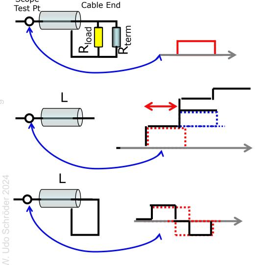
Receiver input impedance  $R_{load} \neq Z_0$ ,  $\rightarrow$  use additional Ohmic termination in parallel
