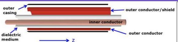
Coaxial cables/transmission lines ←→ traveling waves in cavity resonators
