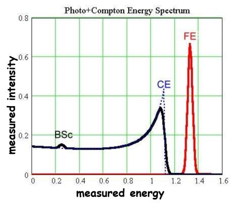
The energy  $E_{\gamma}$  of an incoming photon can be  $\approx$ completely converted into charged particles which are all absorbed by the detector,  $\rightarrow$  measured energy spectrum shows only the full-energy peak (FE, red) Example: photo effect with absorption of struck  $e^-$
