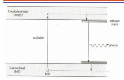
Primary ionization and excitations of solid-state **crystal lattice**: NaI (Tl) = single crystals with well defined periodic lattice  $N \sim 10^{23}$
