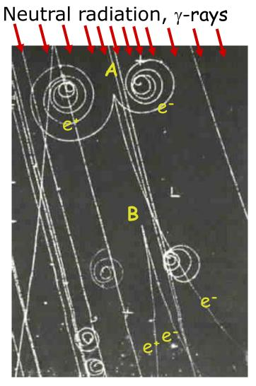
{e+, e-,e-} triplet and one doublet in liquid-H bubble chamber
